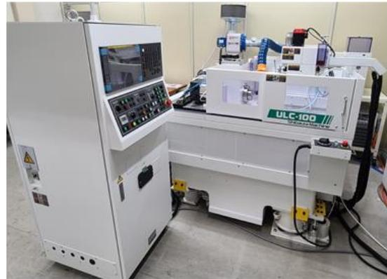
**Fig. 1** Ultra-precision cutting machine (ULC-100D, Shibaura machine Co., Ltd.)
